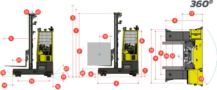
This compact truck features two rear wheel drive and dynamic 360° steering rotation. This contributes to faster procedures for manufacturing distribution and logistics operations.
